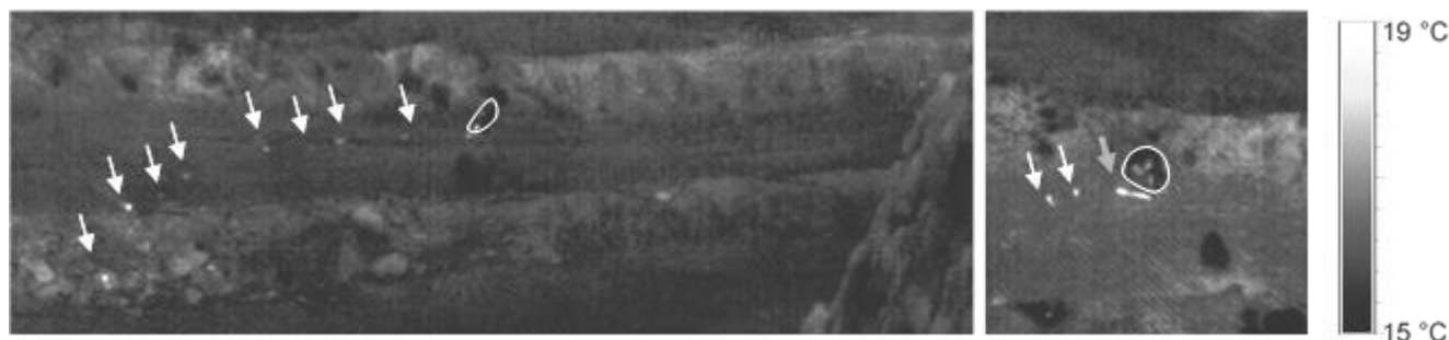
Figure 2: Propagation of a block (white circles) recorded with a thermal camera. Left: illustration of the augmentation of temperature due to rock impacts (white arrows). Right: difference between a bouncing (white arrow) and sliding (grey arrow) impact.
