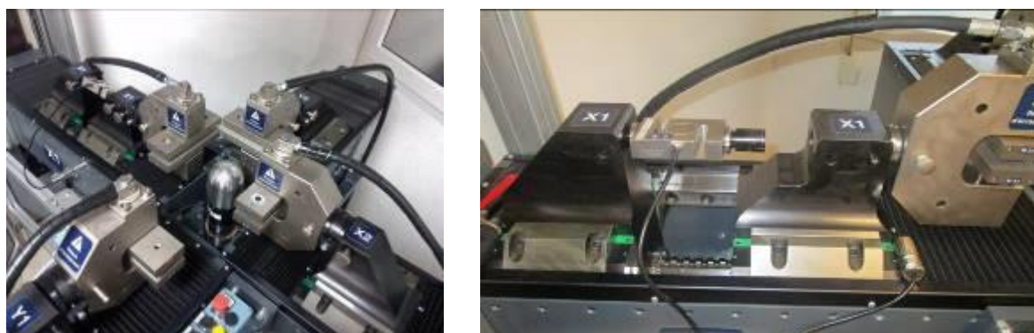
Fig.1 – Tri axial dynamometer: X Y and Z axes
