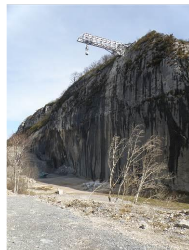
Figure 2: The Ifsttar's impact test device
