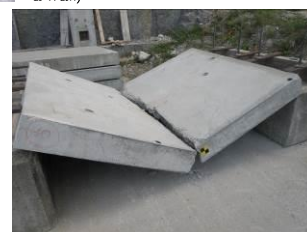
Figure 3: Punching failure (rear face of a wall)
