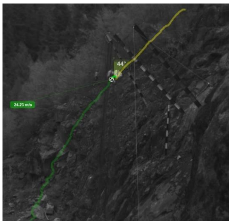
Figure 8 (left): High speed velocity analysis by tracking the block's trajectory through time
