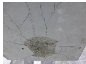
Figure 3: Punching failure (rear face of a wall)
