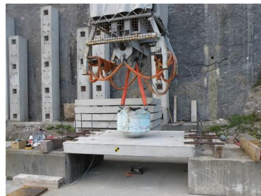
Figure 1: Example of a tested unreinforced concrete wall
