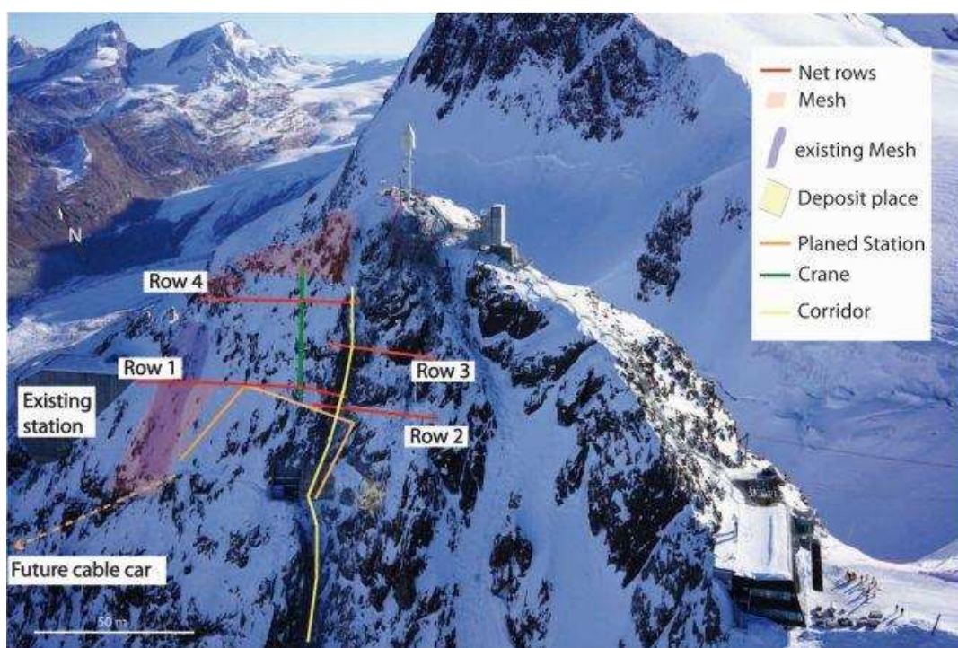
Figure 1: Frontal overview of the west face of the Klein Matterhorn with projected infrastructures and protective measures
